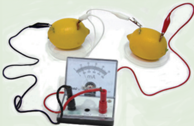
Fig 12.6: Two simple cells connected in series
