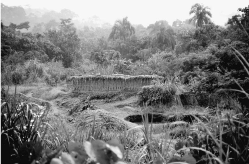
Because of ample rainfall, southern Uganda is characterized by lush vegetation. Bricks, such as these that are being dried before being kilned, are a common housing construction material in the country. Courtesy of Earl P. Scott.
