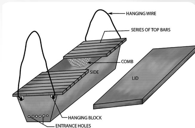
Procedure for constructing a top bar hive
